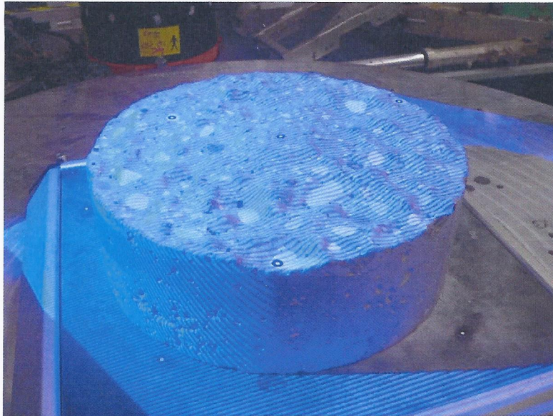
Fig. 3. Concrete specimen during scanning.
